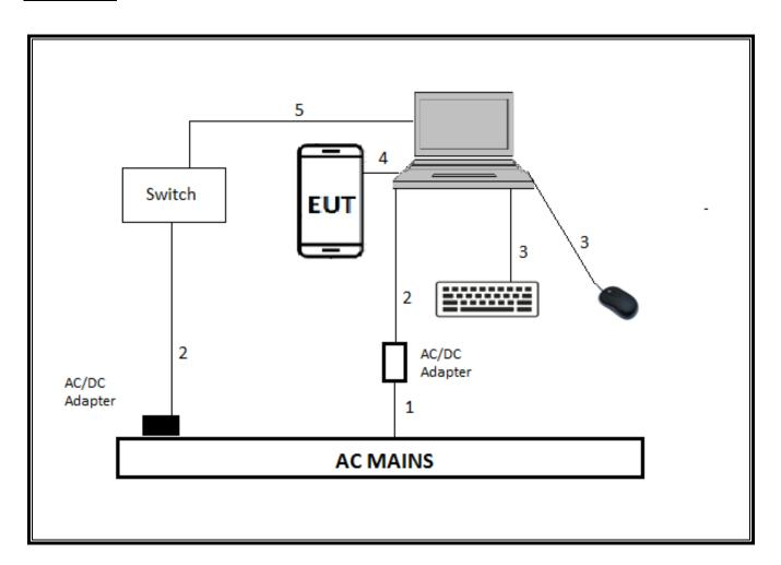
NOTE: Switch location is outside chamber (located in the control room).
