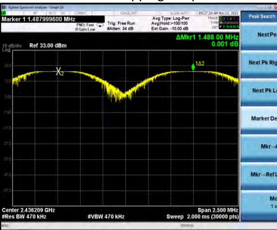
280k Hopping Frequency Separation = 1.5 MHz
