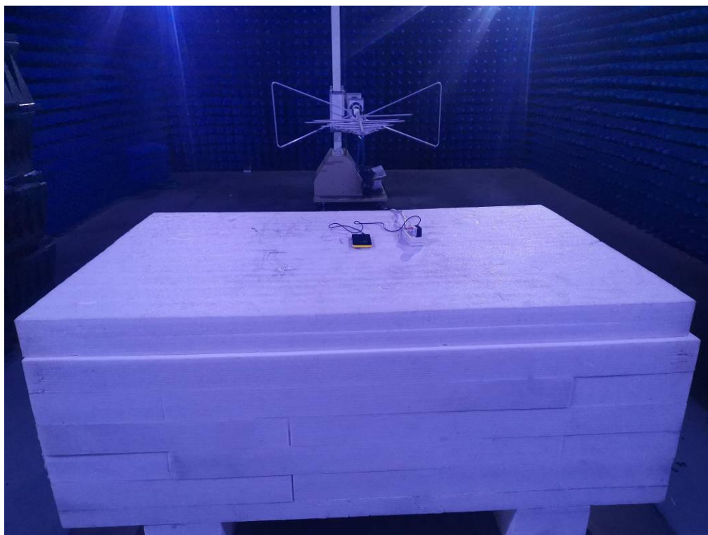
Photo of Radiated Emission Measurement (Above 1G)
