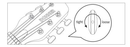
Facing the front tuning peg of the guitar, clockwise rotation can make the strings loose, and counterclockwise rotation can make the strings tight.
