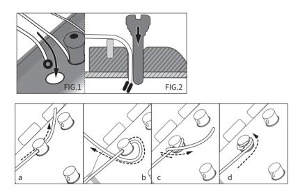
①At first, please put the new string into the bridge hole and the ball end of the string should be put into the hole about 1-2 inches deep (As shown in FIG.1).
