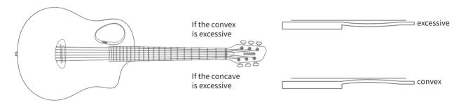
①Please make any adjustments gradually. We suggest that the adjustment time should be completed within 5-10 minutes, and make sure to check the curvature after each 1/2 turn of the truss rod nut.
