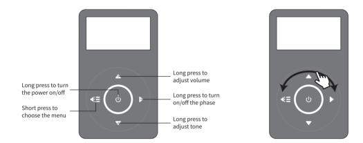
Slide clockwise and counterclockwise can adjust options
