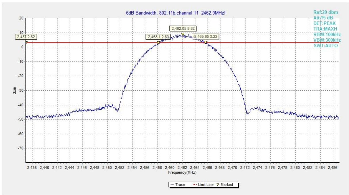
Fig.A.4.3 Occupied 6dB Bandwidth (802.11b, Ch 11)
