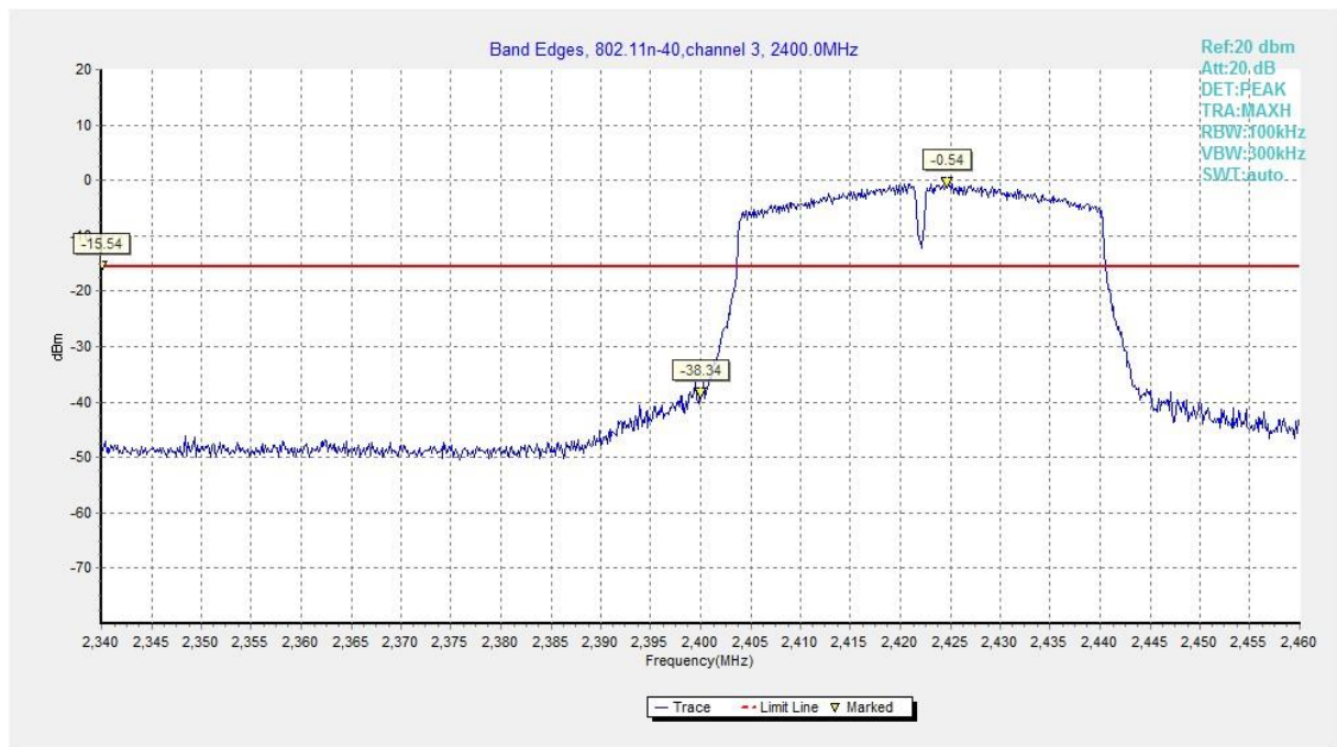
Fig.A.5.7 Band Edges (802.11n-HT40, Ch 3)
