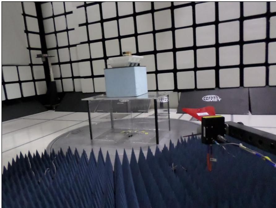
**Photograph 11. Bandedge Testing Antenna**
