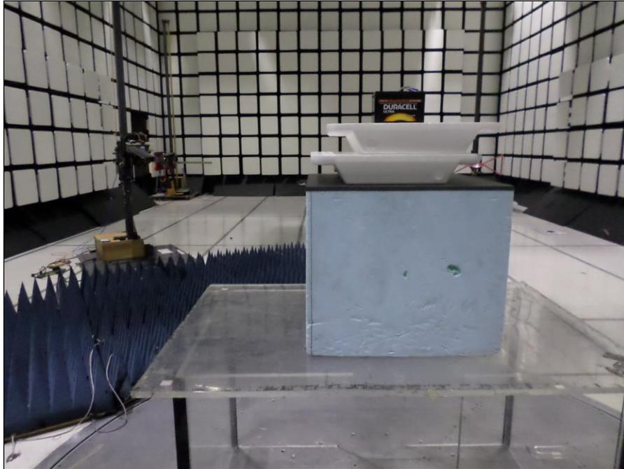
**Photograph 10. Radiated Emissions, Setup Above 1 GHz, Rear**
