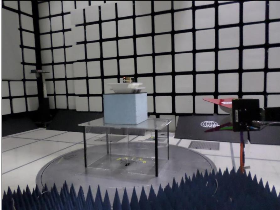
**Photograph 8. Radiated Emissions, Setup Above 1 GHz, Antenna**
