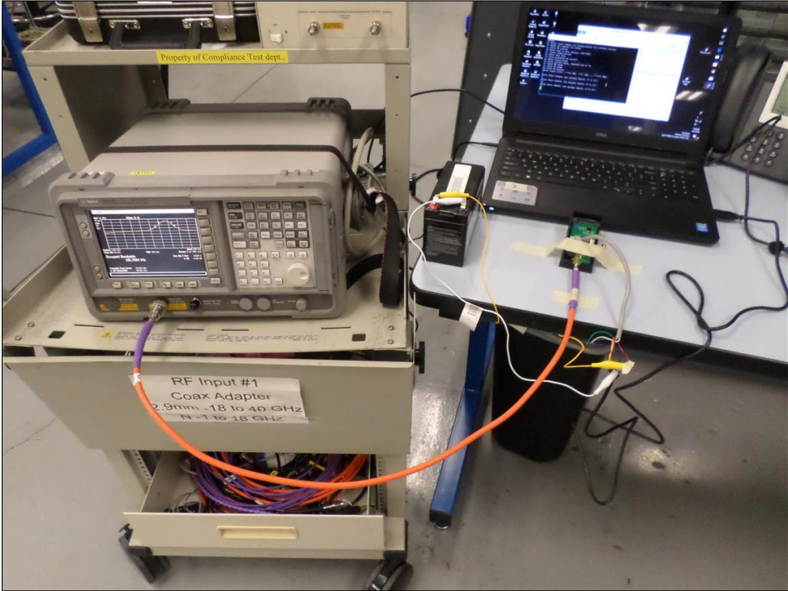
**Photograph 3. Occupied Bandwidth, Conducted Testing Setup**
