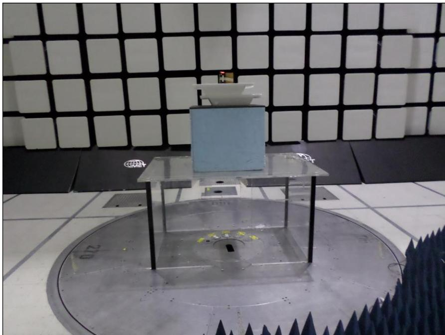
**Photograph 9. Radiated Emissions, Setup Above 1 GHz, Front**
