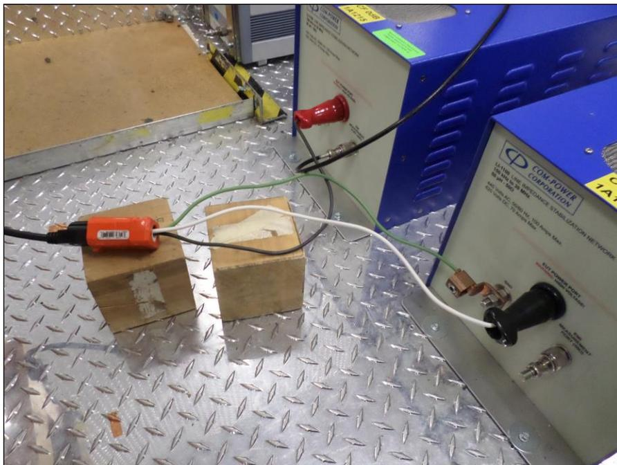
**Photograph 2. Conducted Emissions, 15.207(a), LISN Setup**
