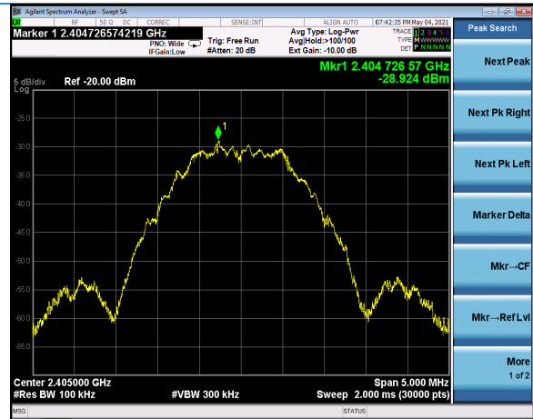
Neg40dBm, channel 11, reference plot -28.9 dBm
