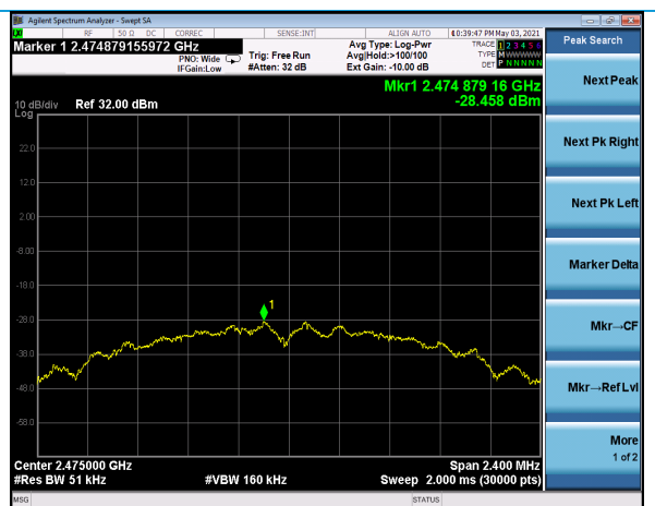
PSD, Channel 25, neg40dBm
