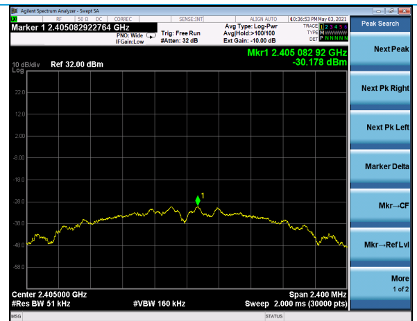
PSD, Channel 11, neg40dBm
