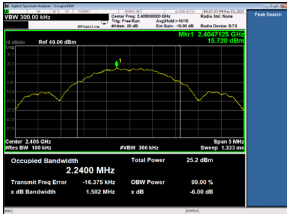
DTS BW, Channel 11, neg4dBm
