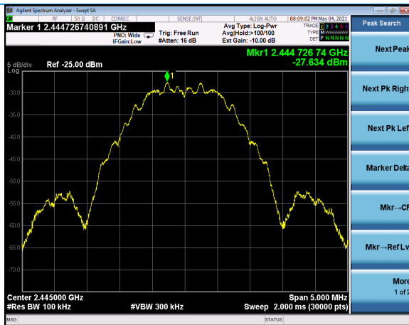
Neg40dBm, channel 19, reference plot -27.6 dBm
