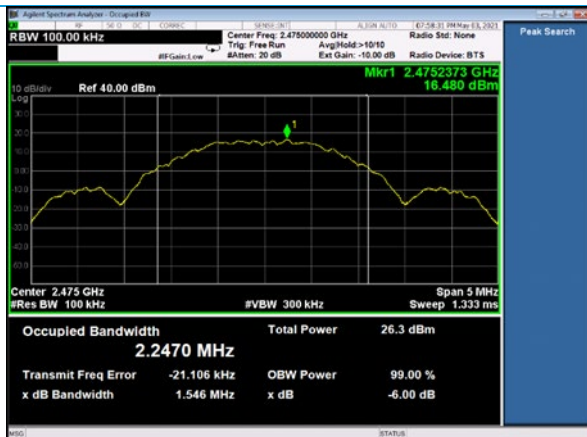
DTS BW, Channel 25, neg4dBm
