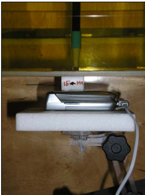
Figure 31: Positional Photograph of the Sagem MC2004a Handset Front Facing Phantom 15mm from the Phantom with Simple Hands Free Accessory (SAR Body Test)
