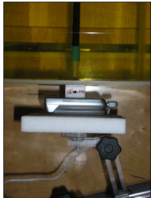
Figure 32: Positional Photograph of the Sagem MC2004a Handset Rear Facing Phantom 15mm from the Phantom with Simple Hands Free Accessory (SAR Body Test)
