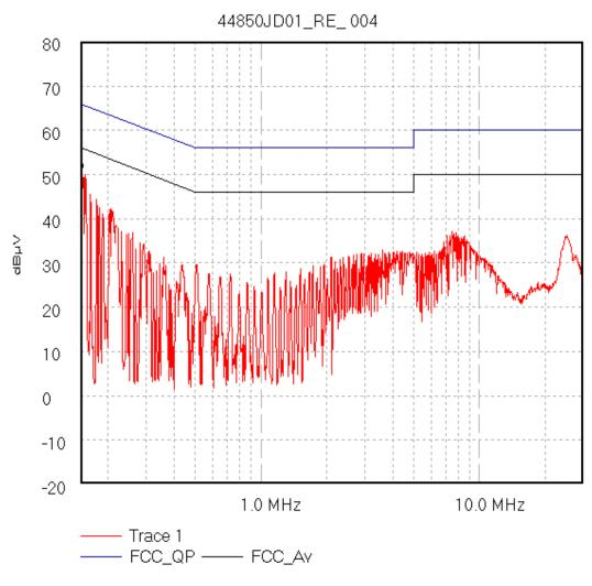
Start 150.0 kHz; Stop 30.0 MHz - Log Scale Ref 80 dBµV; Ref Offset 0.0 dB; 10 dB/div
