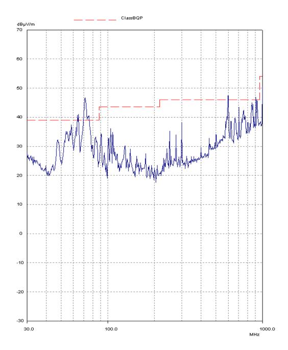
RBW: 120 kHz; VBW: 100 kHz; Att 0 dB; Swp: Coupled
