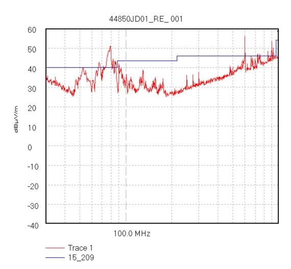
Start 30.0 MHz; Stop 1.0 GHz - Log Scale Ref 60 dBµV/m; Ref Offset 0.0 dB; 10 dB/div
