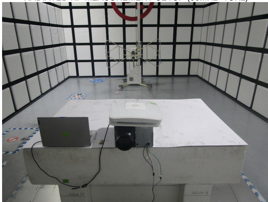
RADIATED RF MEASUREMENT SETUP (Below 30MHz)
