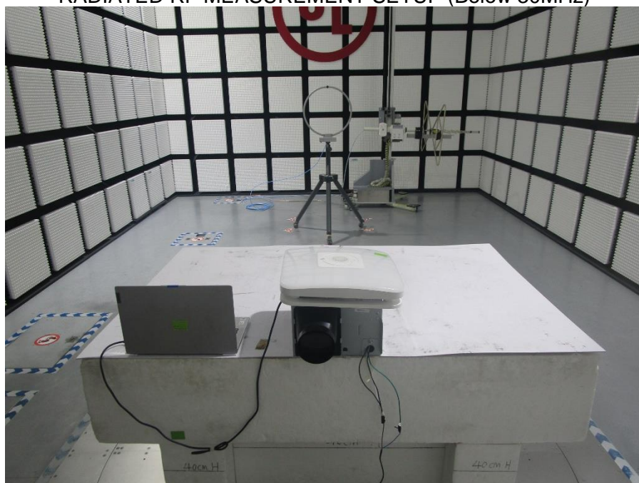
RADIATED RF MEASUREMENT SETUP (Below 30MHz)
