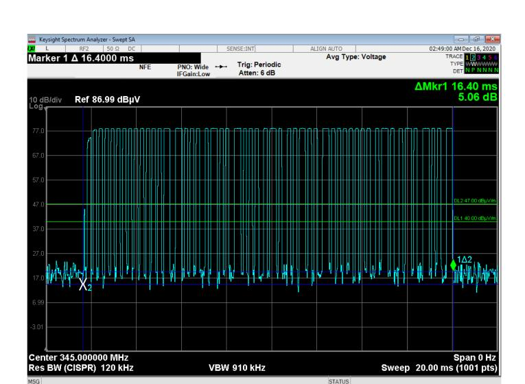
First Pulse = 1 = (1\*23.2 us) = 23.2 usNumber of Small Pulses = 41 = (41\*148 us) = 6068 usNumber of Large Pulses = 11 = (11\*283 us) = 3113 us
