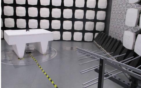
1.2 Radiated Emissions(9kHz-30MHz) Test Setup
