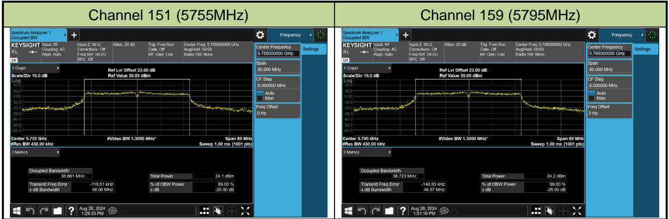
802.11ac-VHT80 26dB Bandwidth & 99% Bandwidth
