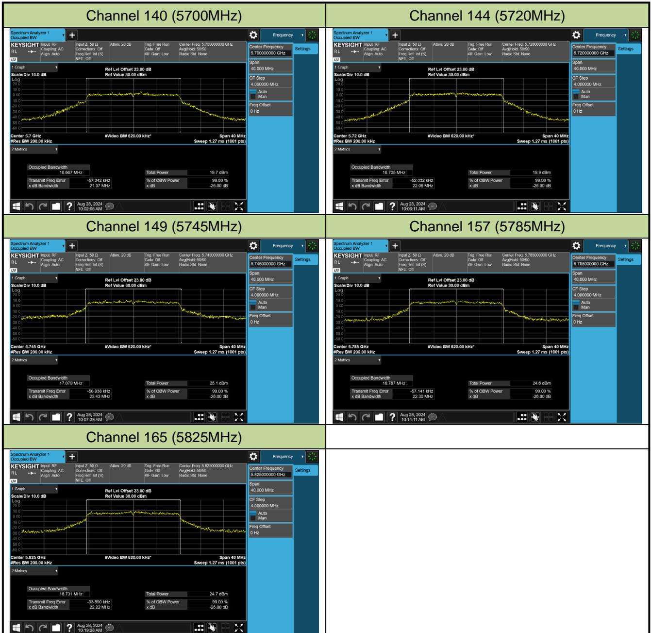
802.11ac-VHT20 26dB Bandwidth & 99% Bandwidth
