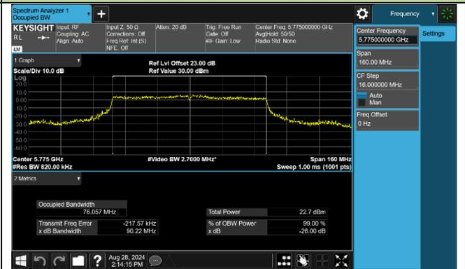
802.11ac-VHT160 26dB Bandwidth & 99% Bandwidth
