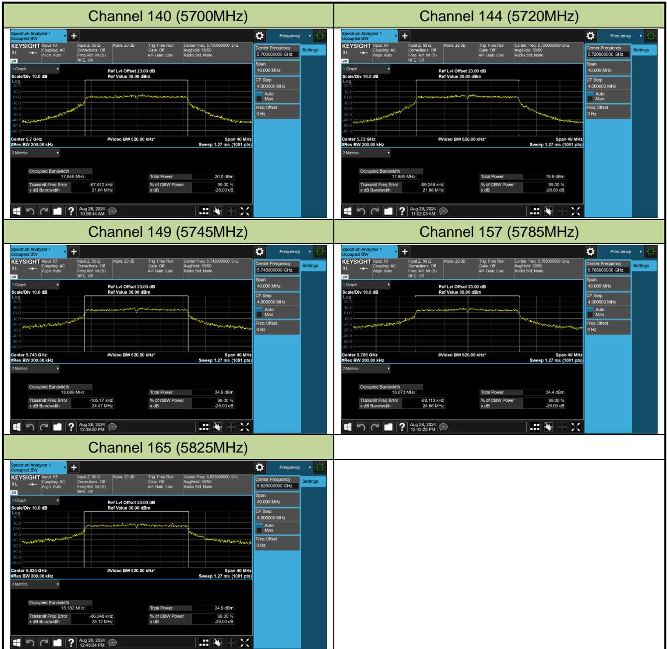
802.11ac-VHT40 26dB Bandwidth & 99% Bandwidth
