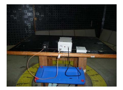
Photograph No.9 Conducted emission on AC power lines test setup
