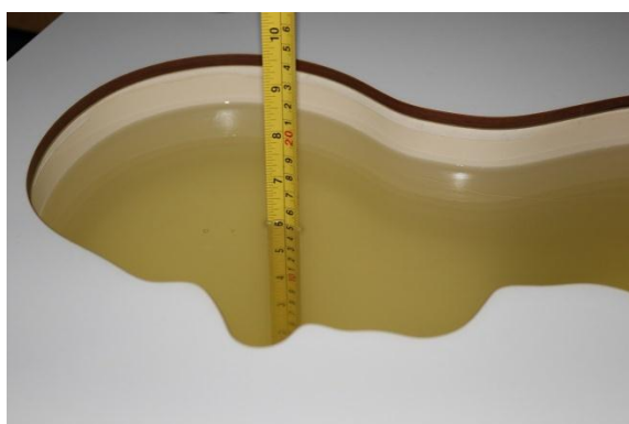
Liquid depth in the head phantom (1750MHz)
