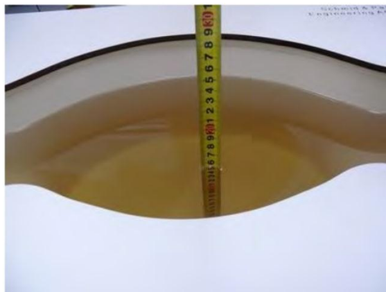
Liquid depth in the body phantom (835MHz)
