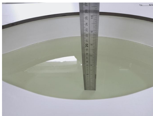
Liquid depth in the body phantom (1900MHz)
