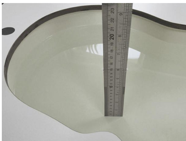
Liquid depth in the head phantom (1900MHz)
