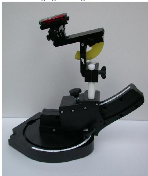
Device holder supplied by SPEAG
