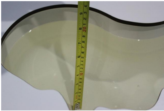
Liquid depth in the head phantom (2600MHz)
