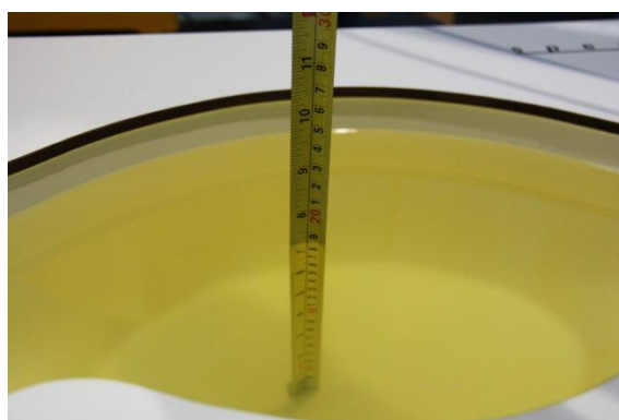
Liquid depth in the body phantom (1750MHz)
