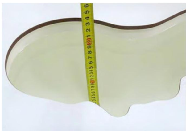
Liquid depth in the head phantom (1900MHz)
