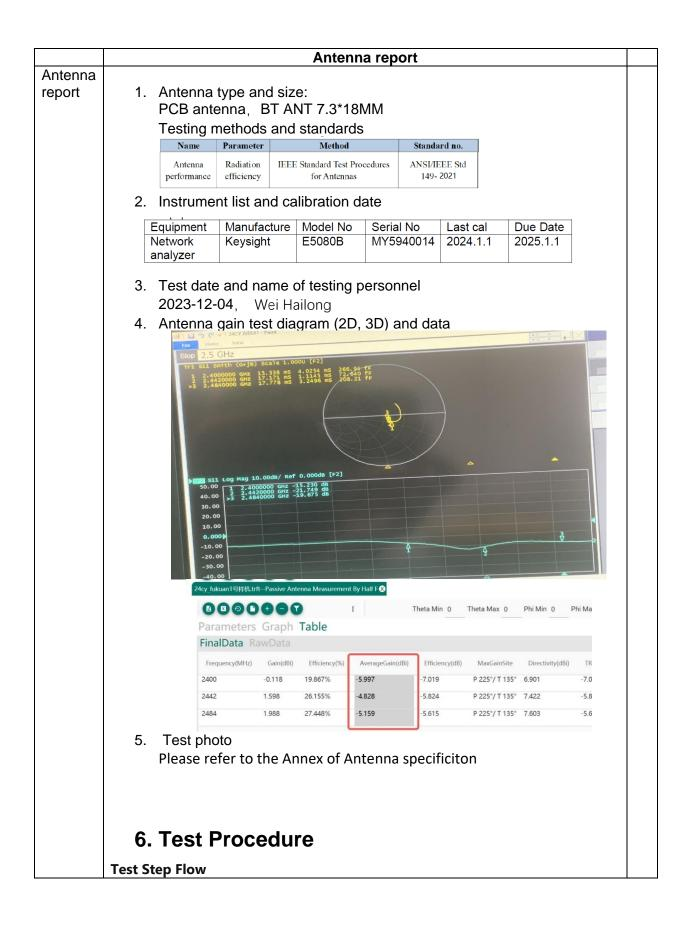
1. Maintain the test ambient temperature of 23t2 C, the instrument is powered on and preheated for more than 30 minutes
