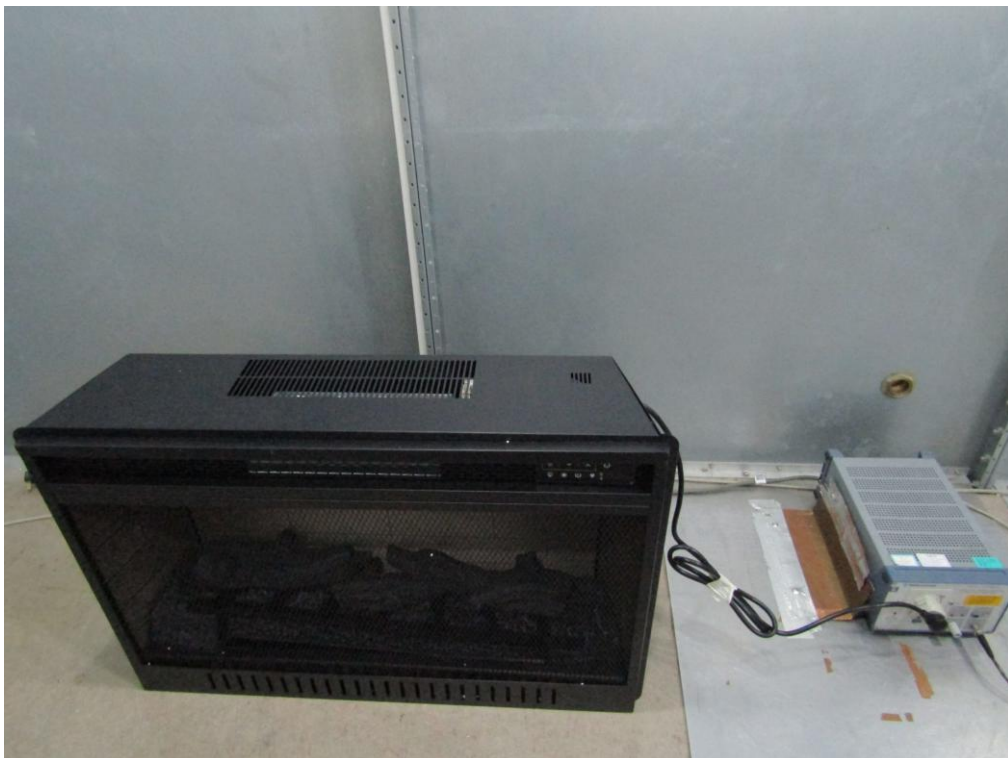
Measurement of Conducted Emission Test Set Up
