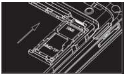
Figure 4-1 Placement of SIM Card
