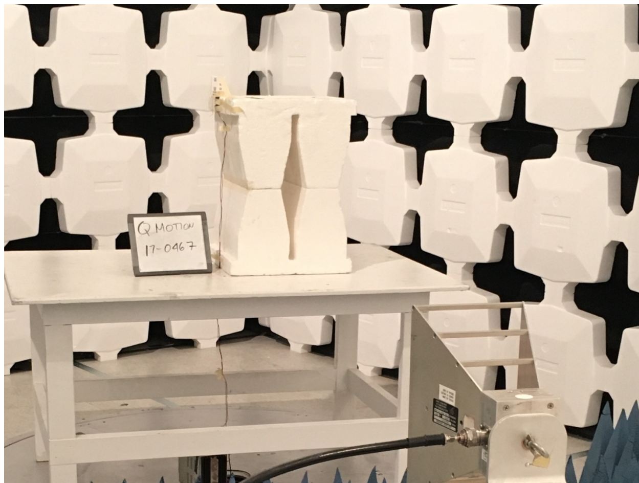
Figure 2. Above 1 GHz, Radiated Emissions Test Setup, Front
