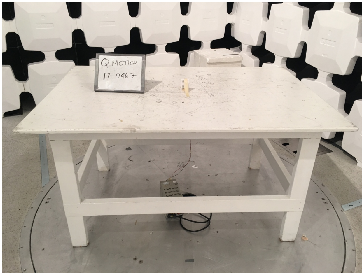
Figure 1. Below 1 GHz Radiated Emissions Test Setup, Front
