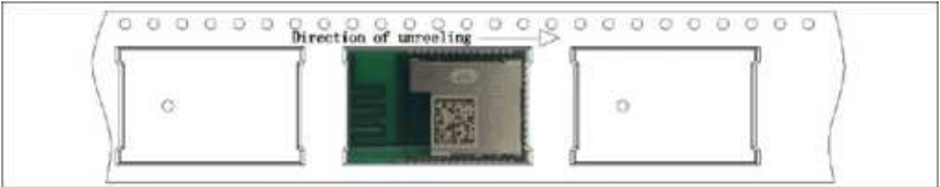
Figure 9 Component orientation in tape and unreeling direction
