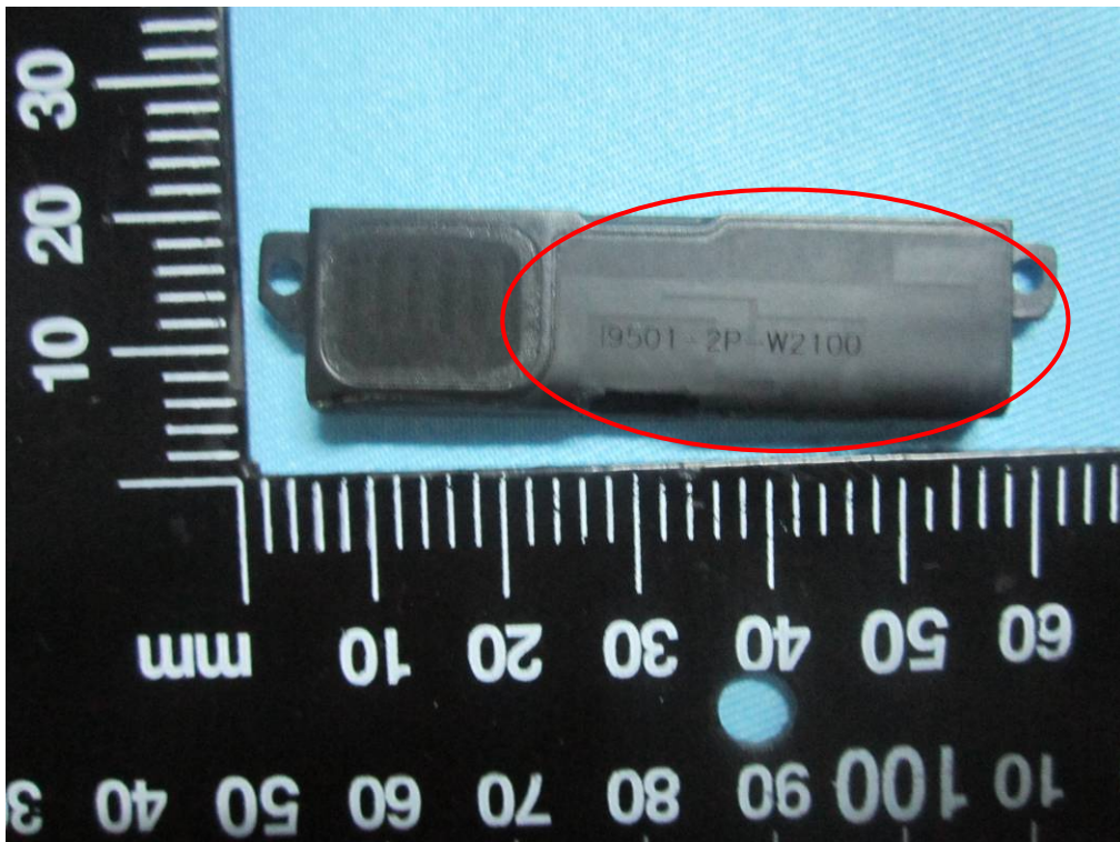
GSM/PCS/UMTS-FDD Antenna View
