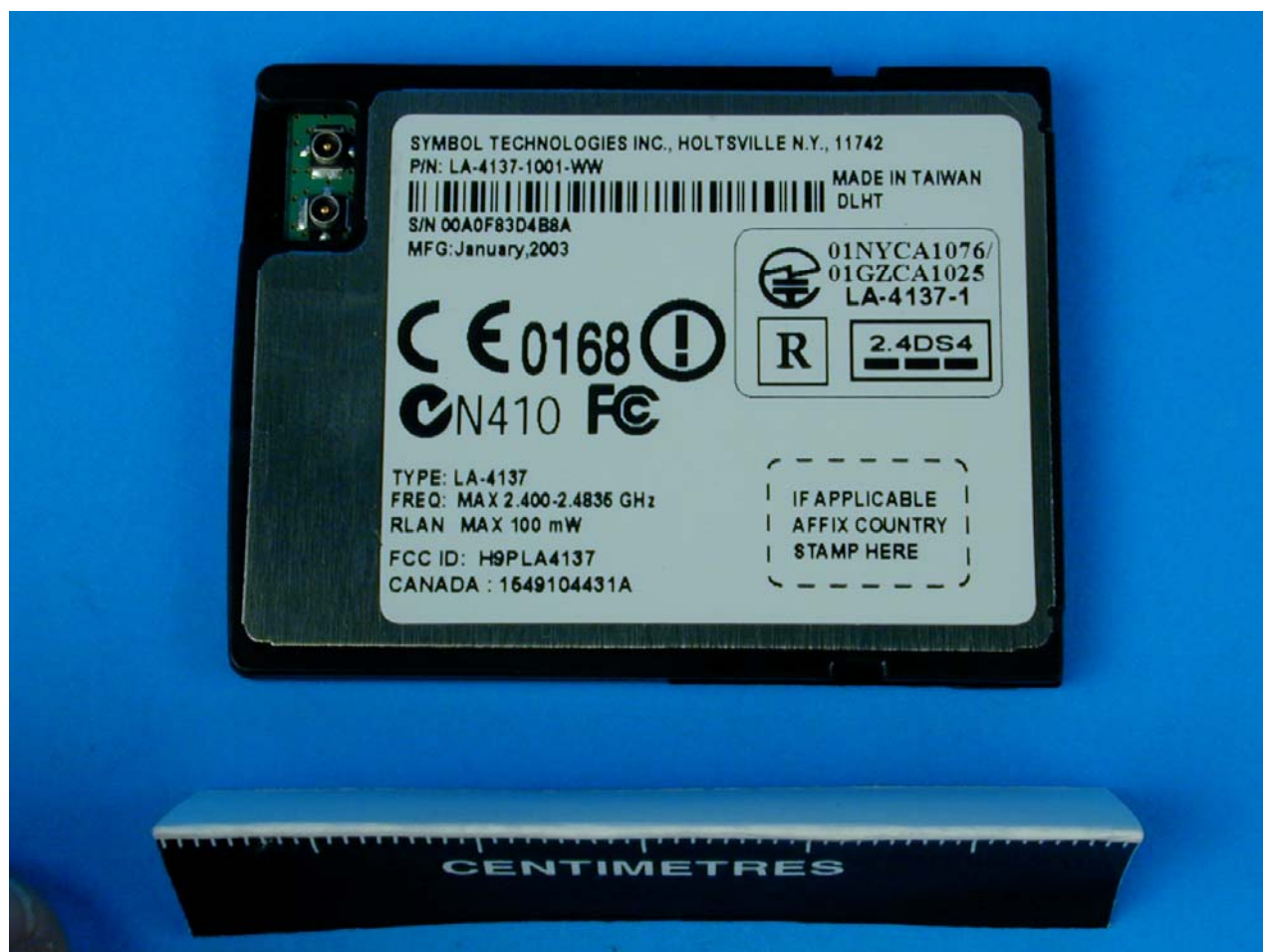
Photograph 15 4111-GPRS View of LA-4137 RLAN Card
