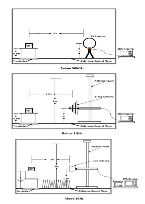
Above 18 GHz shall be extrapolated to the specified distance using an extrapolation factor of 20 dB/decade form 3m to 1m.
