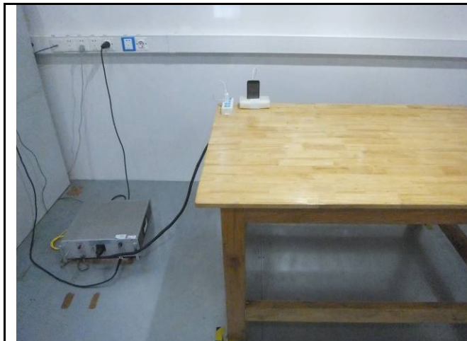
Conducted Emissions Test Setup Front View
