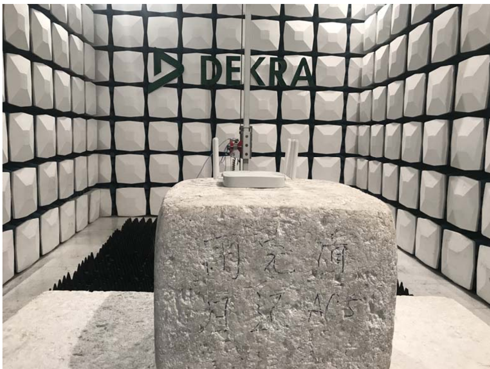
Description: Radiated Emission Test Setup for 1~18GHz
