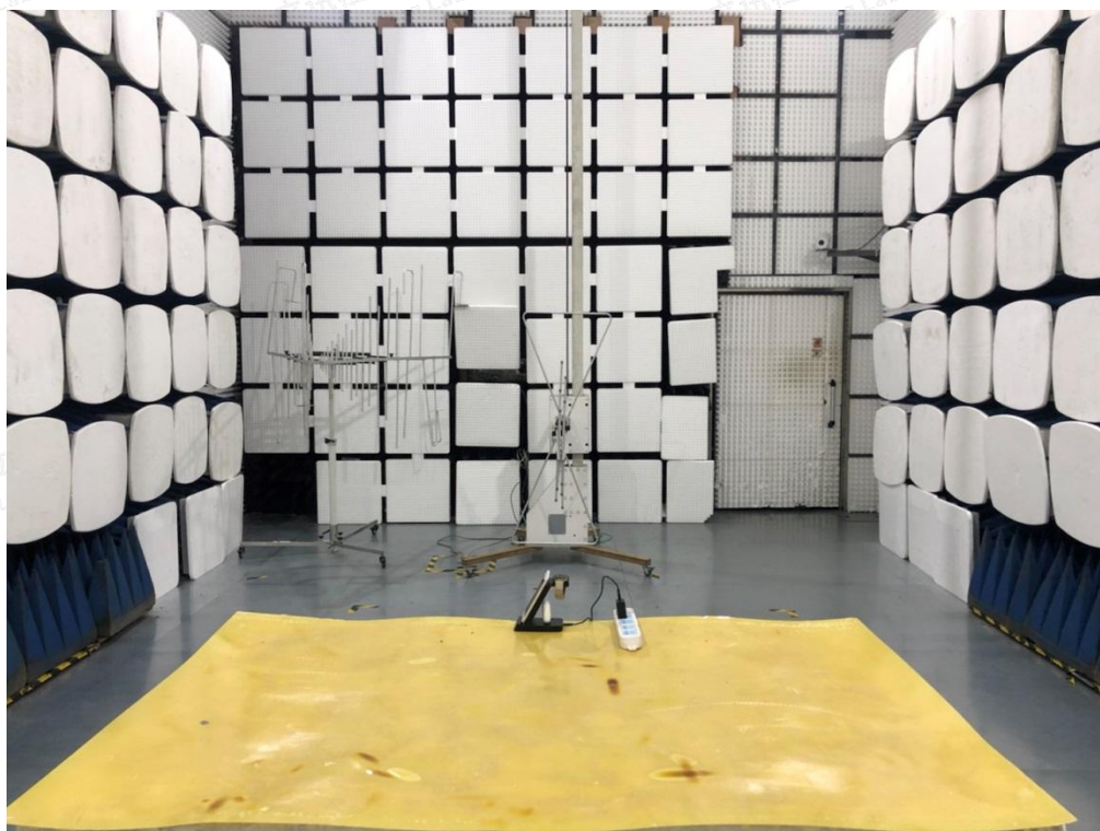
Radiated Emission below 1GHz-AC adapter charge mode
