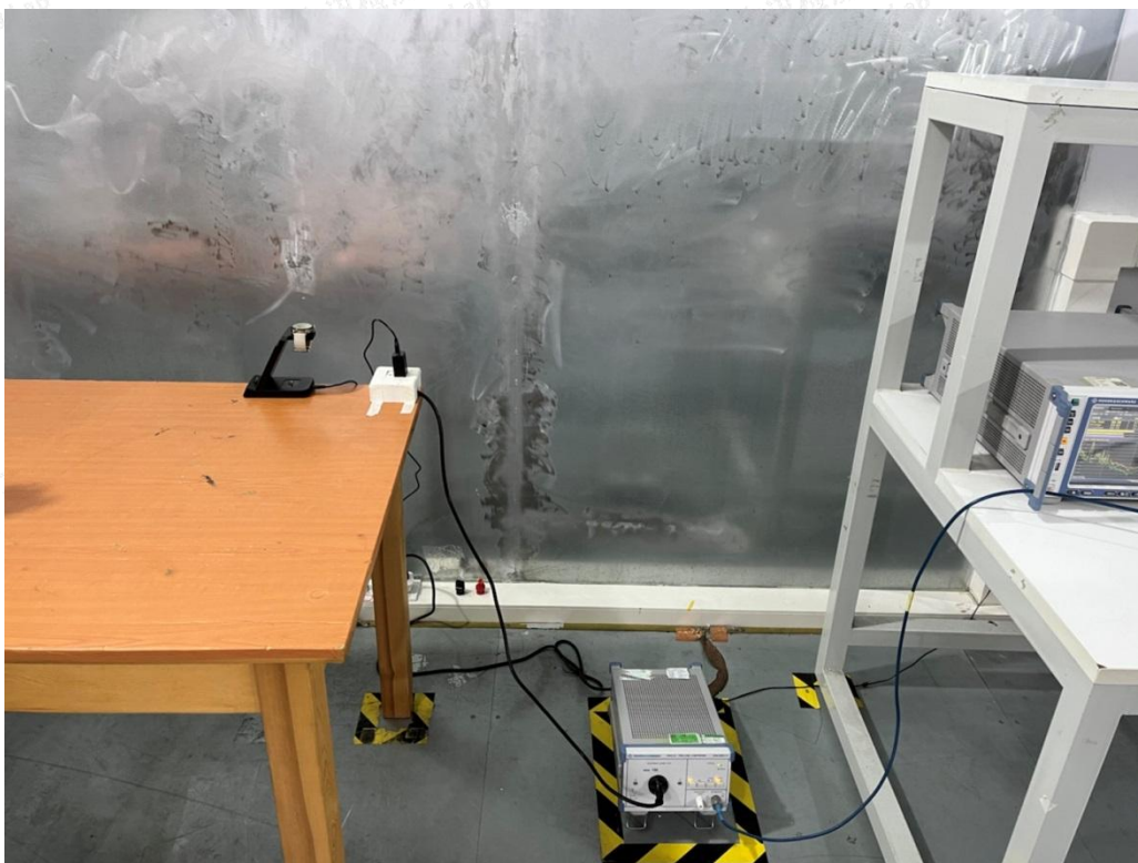
Conducted Emission-AC adapter charge mode
