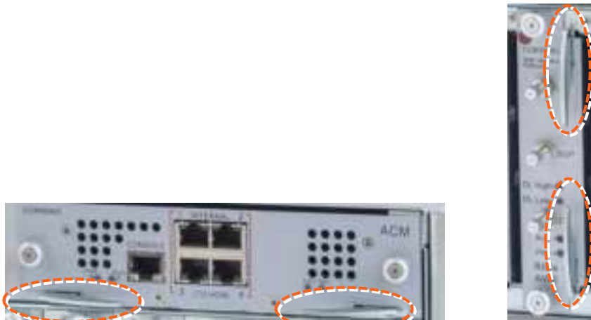
Figure 8: Module Captive Screws and Ejectors
