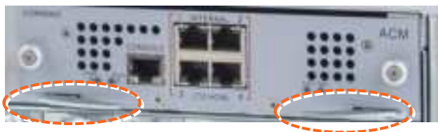
Figure 5: Module Captive Screws and Ejectors
