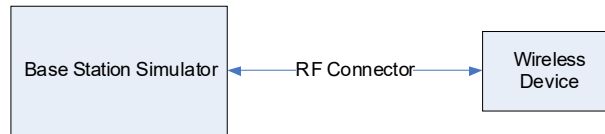
Figure 9-2 Power Measurement Setup
