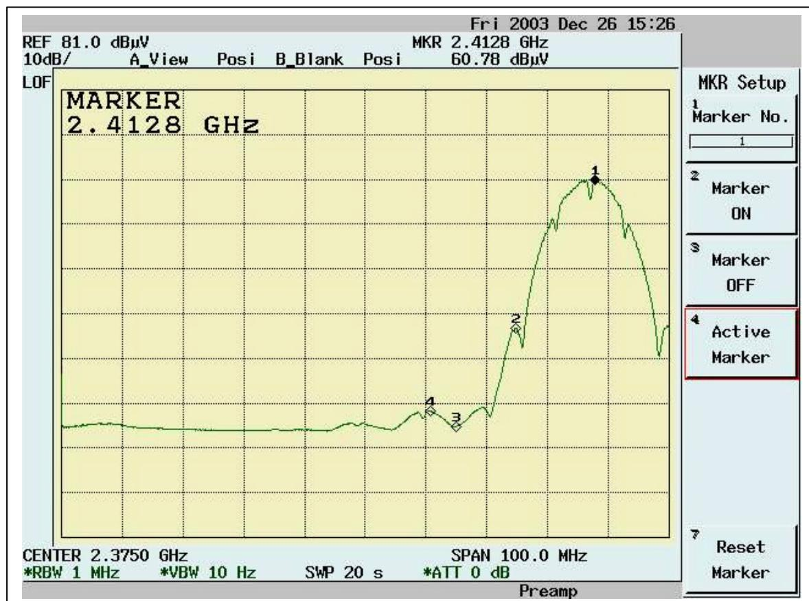
Band Edge measurement for radiated emission in Restricted Band(Radiated)
