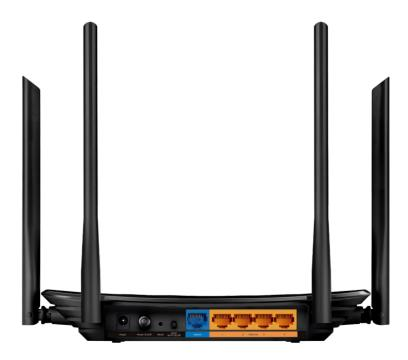
The router's ports (view from left to right) are located on the rear panel.
