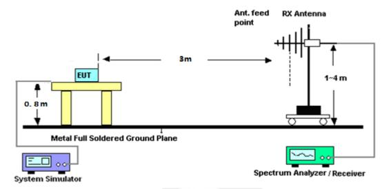
For radiated test from above 1GHz
