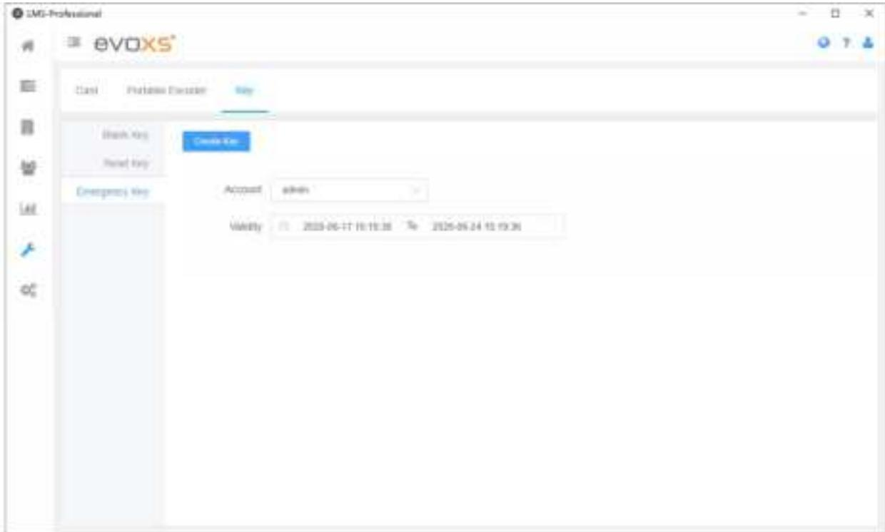
1) Enter the emergency key interface, put the key on the local encoder and click "Create Key". The validity of the emergency key can be customized. Users of the key shall be selected before creating, and the emergency key can only be used by software operators and staffs. The factory key must be registered as the key of the project before it can be created as the emergency key.
