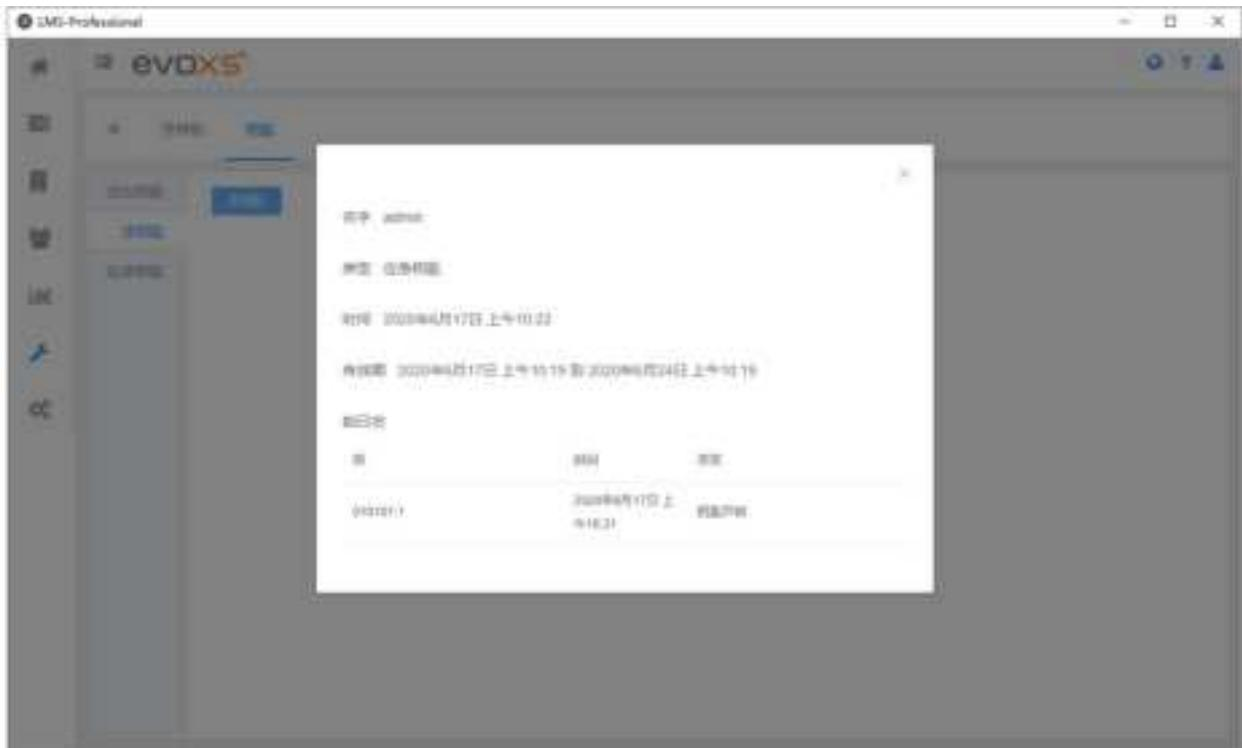
2) Read the basic information of the key in the project. The factory key must be registered as the key of the project before reading. The success event of unlocking is recorded in the key, and the event is read at the same time when reading the key.
