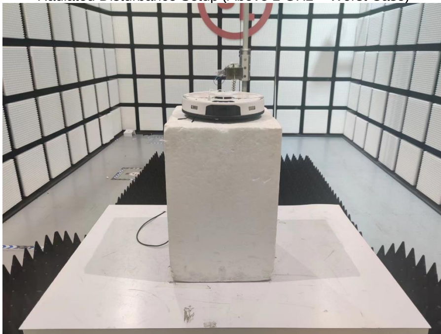
Radiated Disturbance Setup (Above 1 GHz – Worst Case)
