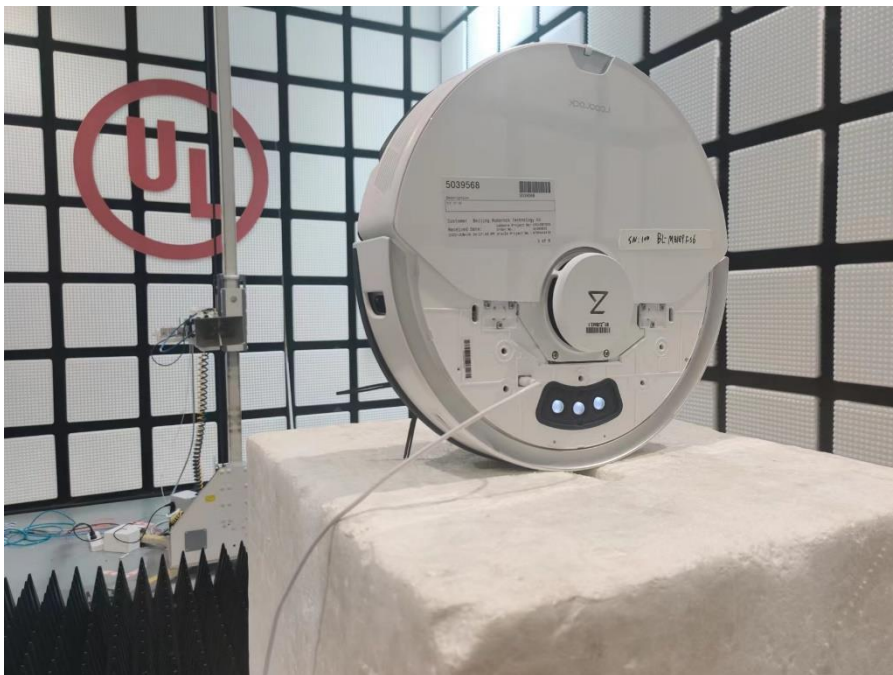
Radiated Disturbance Setup (Above 1 GHz – Y axis)
