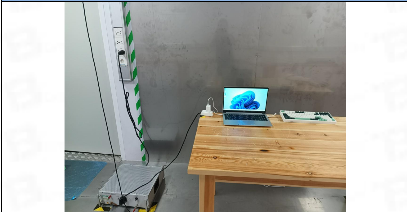
Conducted Emission at AC power line
