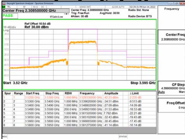
Emission Mask Band48 15MHz QPSK RB75 0 CH55990
