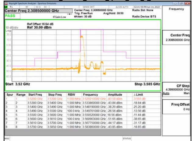
Emission Mask Band48 10MHz QPSK RB1 0 CH55990
