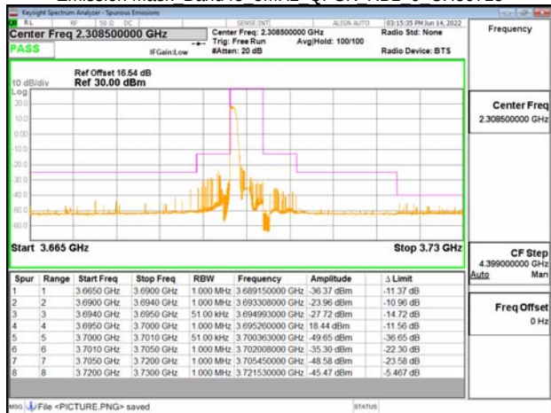
Emission Mask Band48 5MHz QPSK RB1 0 CH56715
