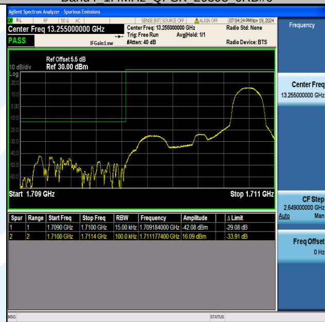
Band4 1.4MHz 16QAM 19957 1RB#5
