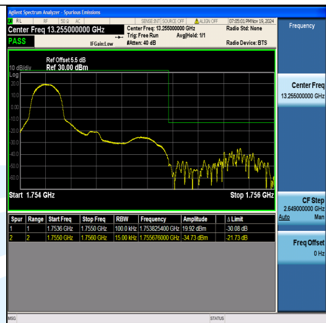
Band4 1.4MHz 16QAM 20393 1RB#0
