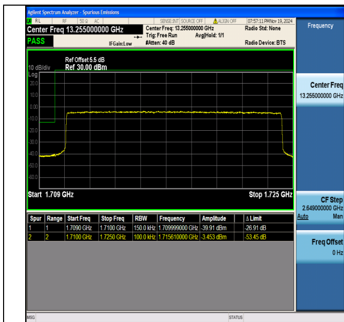
Band4 15MHz 16QAM 20025 75RB#0
