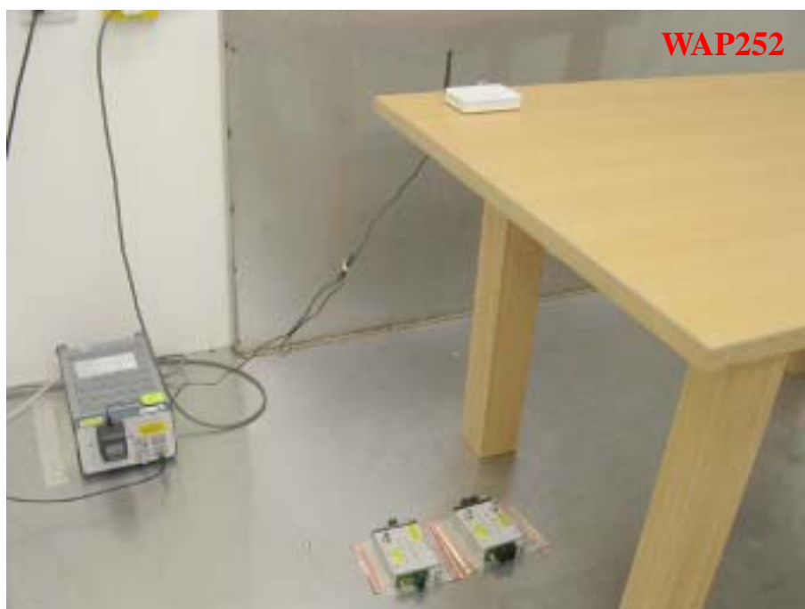
Photo 2: Conducted Emission Test Set-up
