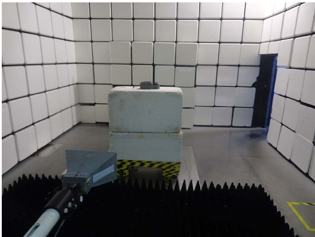
Picture 1: Radiated Spurious Emissions Test setup
