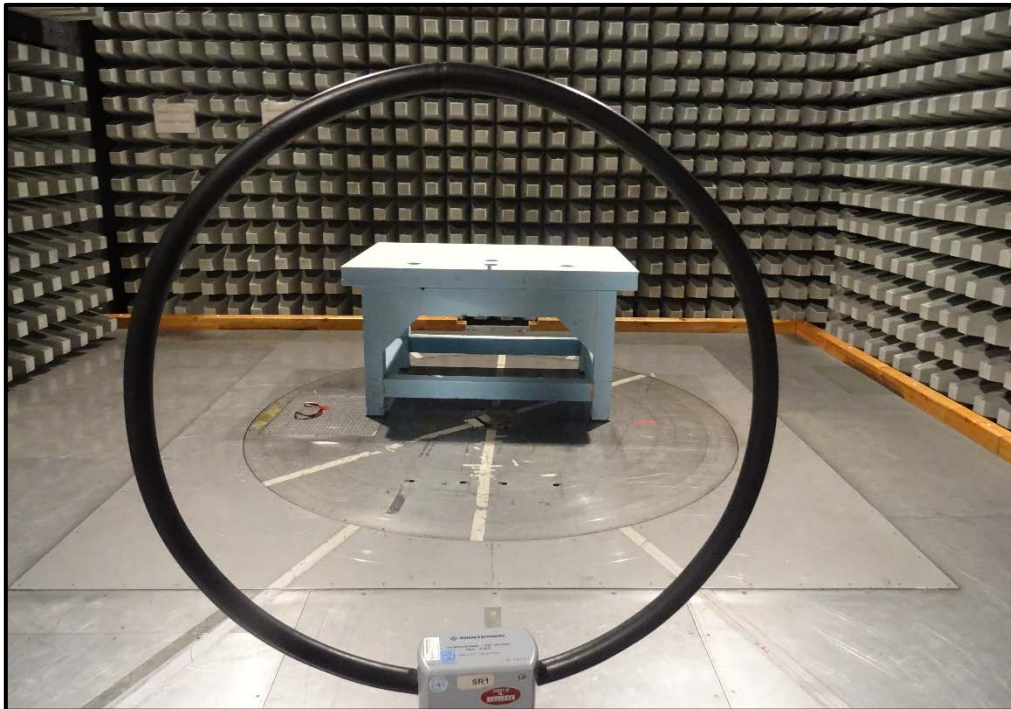
Picture 1 Radiated Test Setup-9 kHz to 30 MHz EUT
