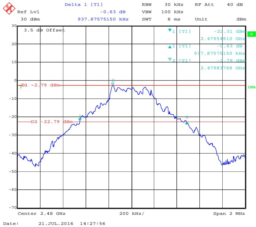
**EDR ( $\pi/4$ -DQPSK): Low Channel**
