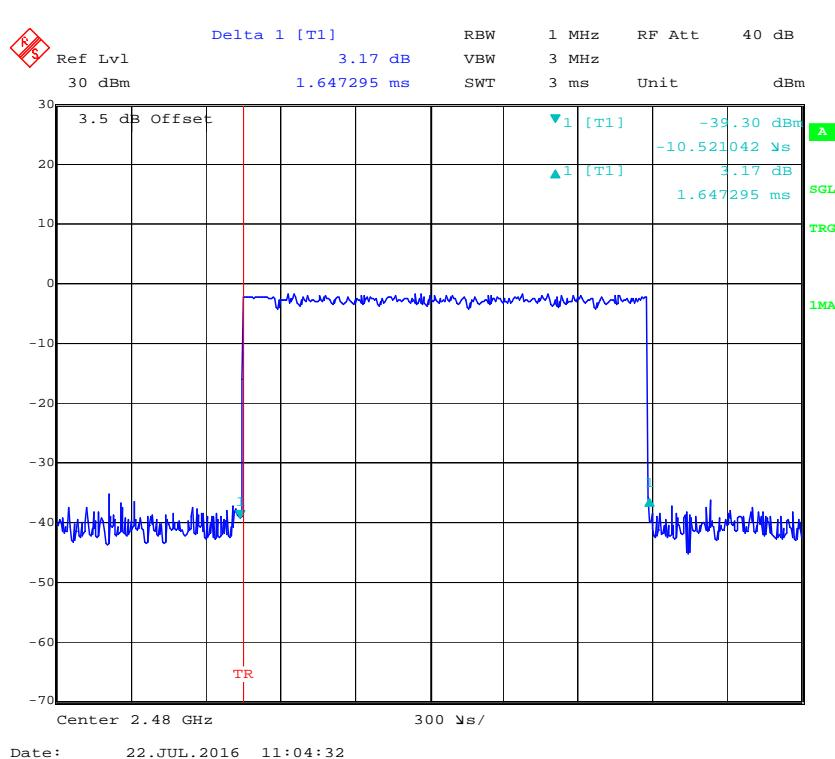
**Pulse time, Low Channel, 3DH5**
