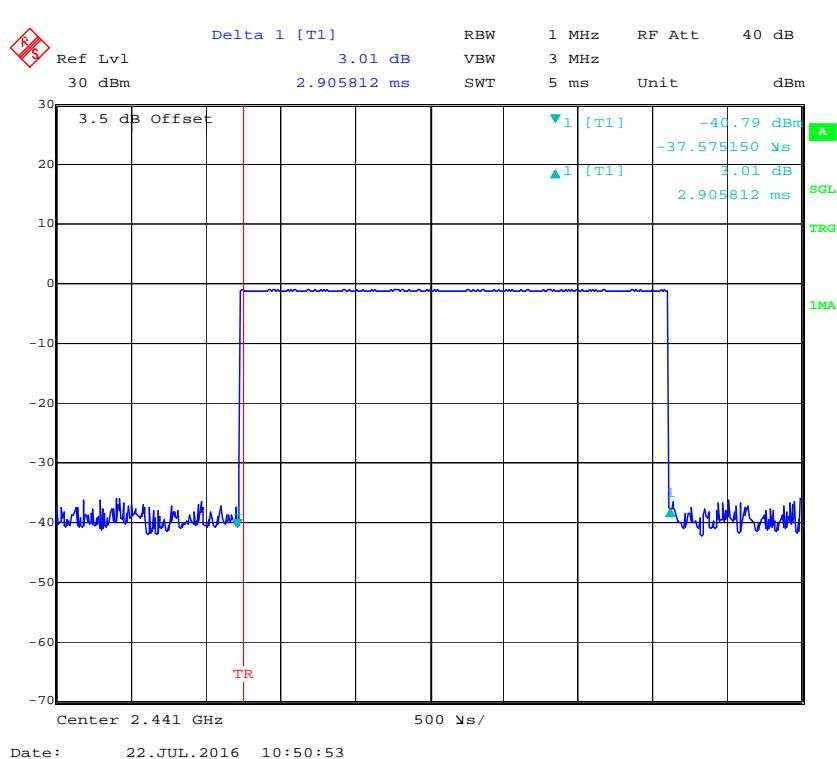
**Pulse time, High Channel, DH5**
