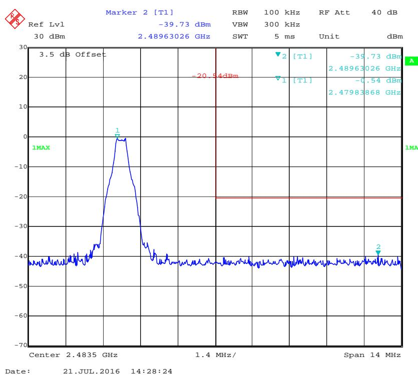
**EDR ( $\pi/4$ -DQPSK): Band Edge-Low**
