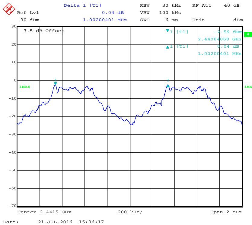
**BDR (GFSK): High Channel**
