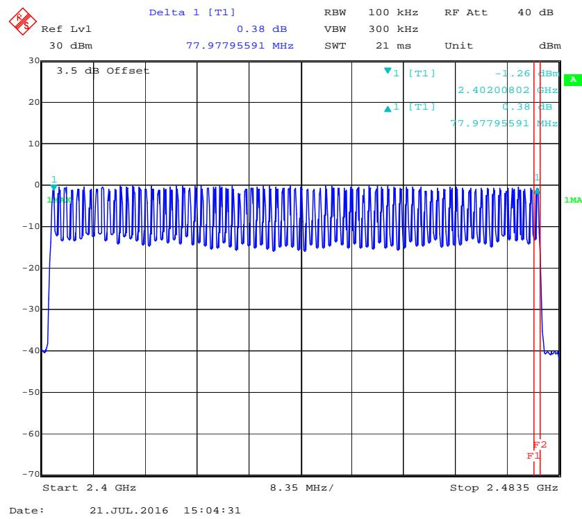
**EDR ( $\pi/4$ -DQPSK): Number of Hopping Channels**
