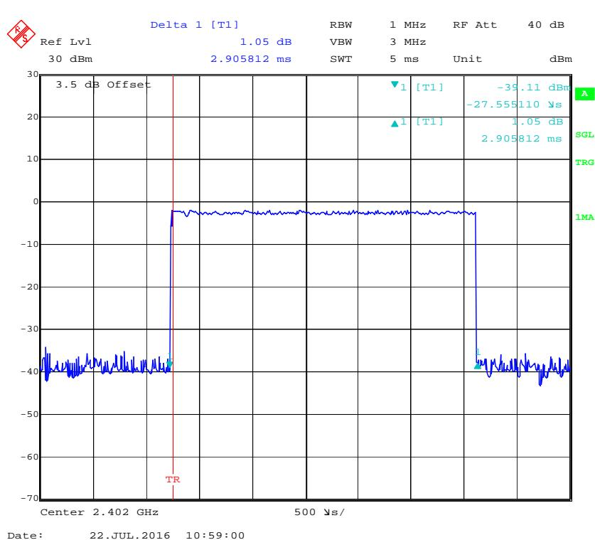
**Pulse time, Middle Channel, 2DH5**
