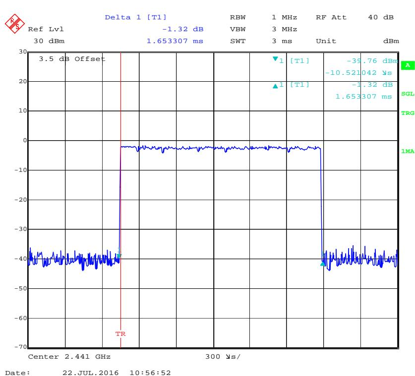
**Pulse time, High Channel, 2DH3**
