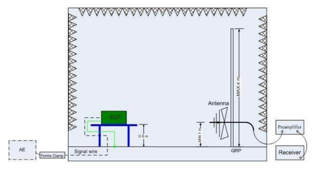
Radiated tests above 1GHz
