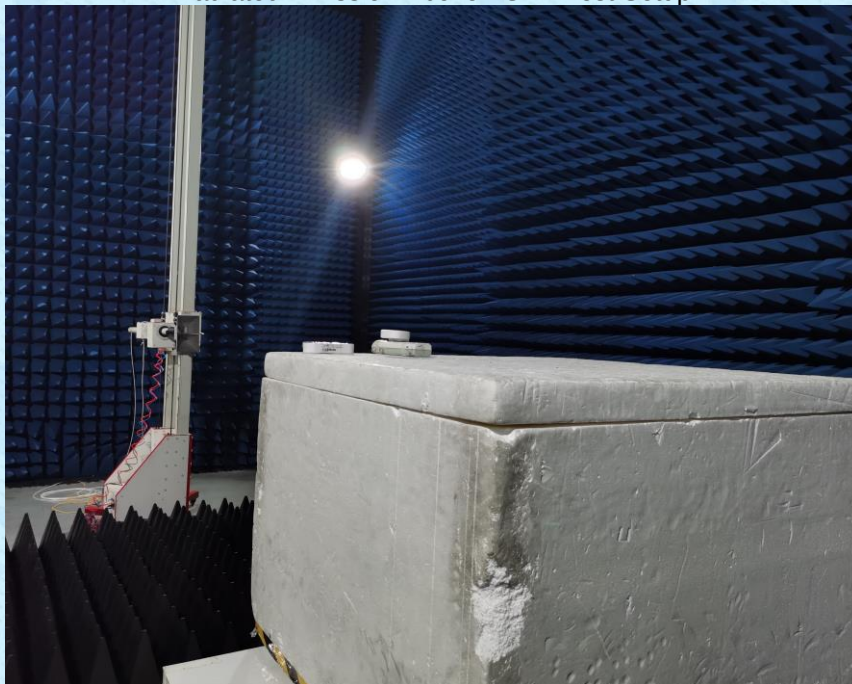
Radiated Emission Above 1GHz Test Setup
