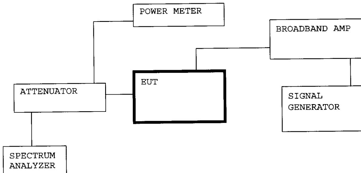
RF power was measured with a HP power meter. Power output was 30 Watts (44.77dBm). Power output was check for low, middle, high channel.
