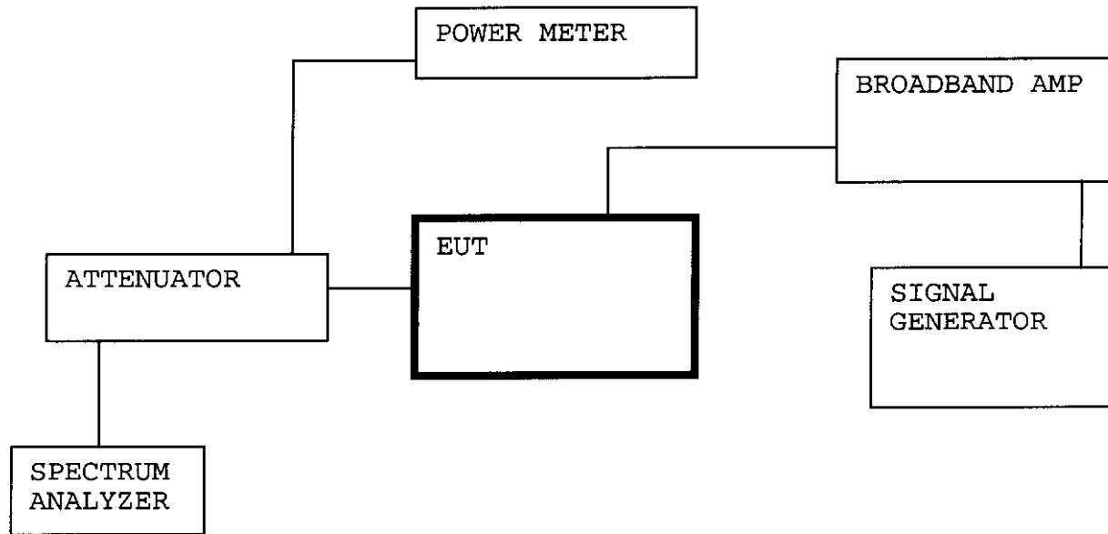
Section 90.205 refers to Section 90.635 were it states that maximum power is 500Watts. RF power was measured with a HP power meter. Power output was 30 Watts (44.77dBm). Power output was check for low, middle, high channel.
