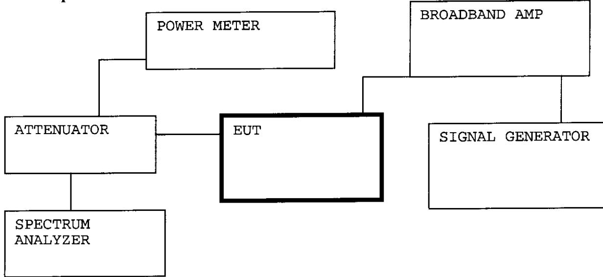
As required in Section 90.209 plots of occupied bandwidth were made one for the output from signal generator and another for output from amplifier. Test result are presented in spectrum analyzer plots from Low to High channels both GSM modulation and CW. Table shows the order of the plots.
