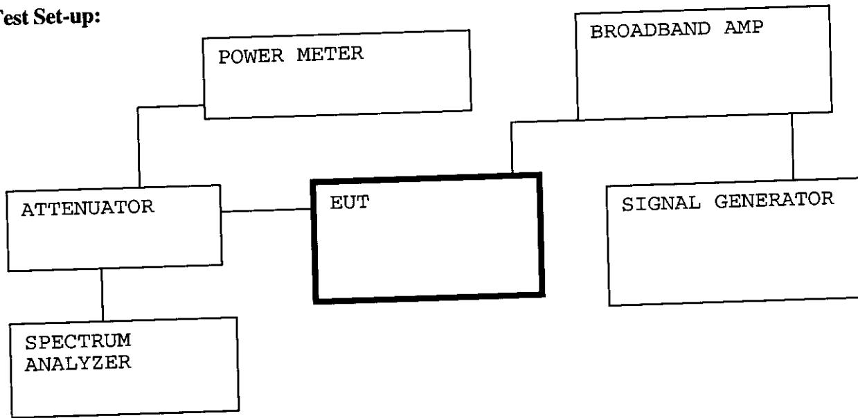
Plots of occupied bandwidth were made one for the output from signal generator and another for output from amplifier. Test results are presented in spectrum analyzer plots from Low to High channels both GSM modulation and CW. Table shows the order of the plots.
