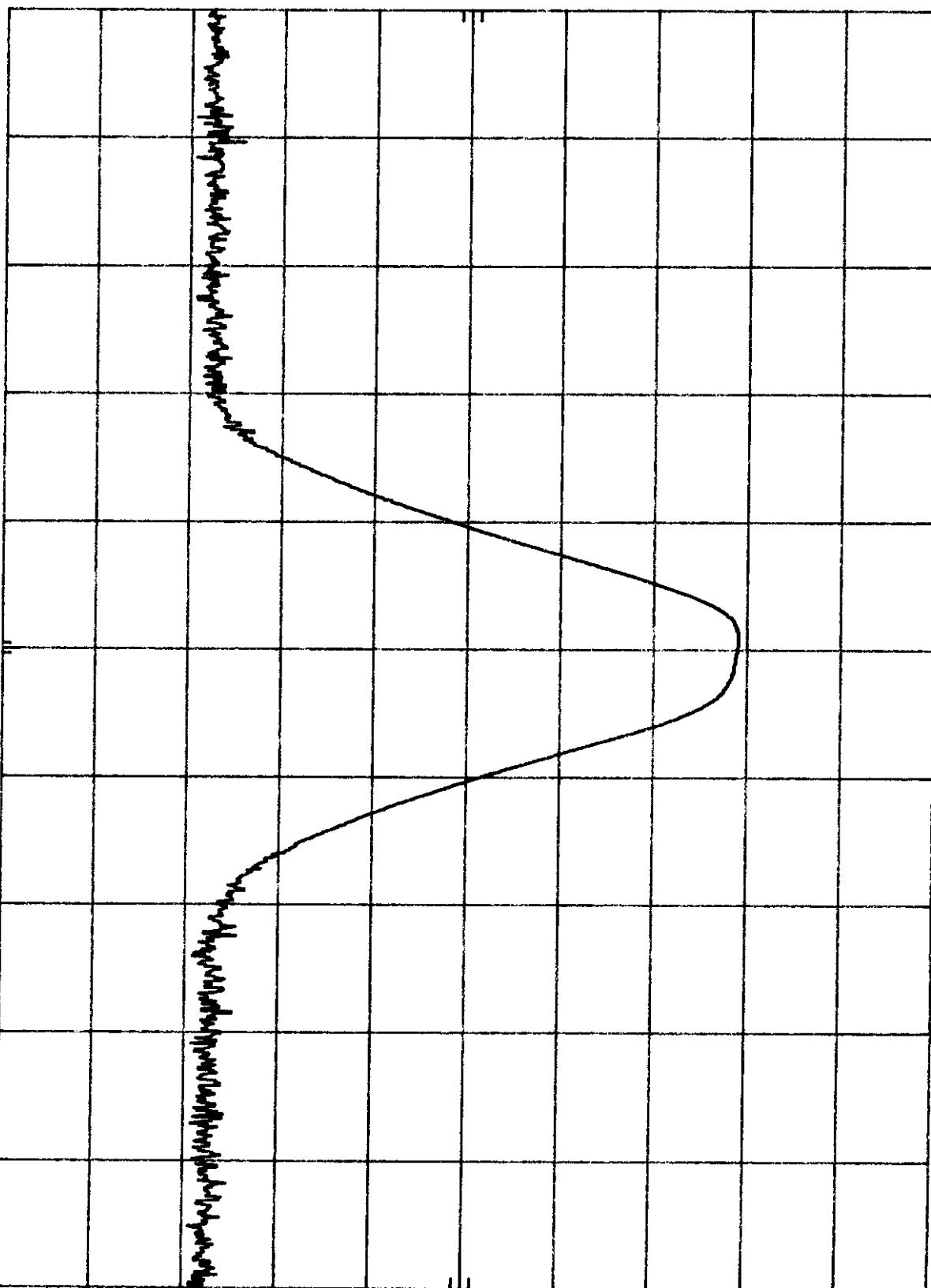
CENTER 940.00 MHz RES BW 100 kHz VBW 100 kHz
