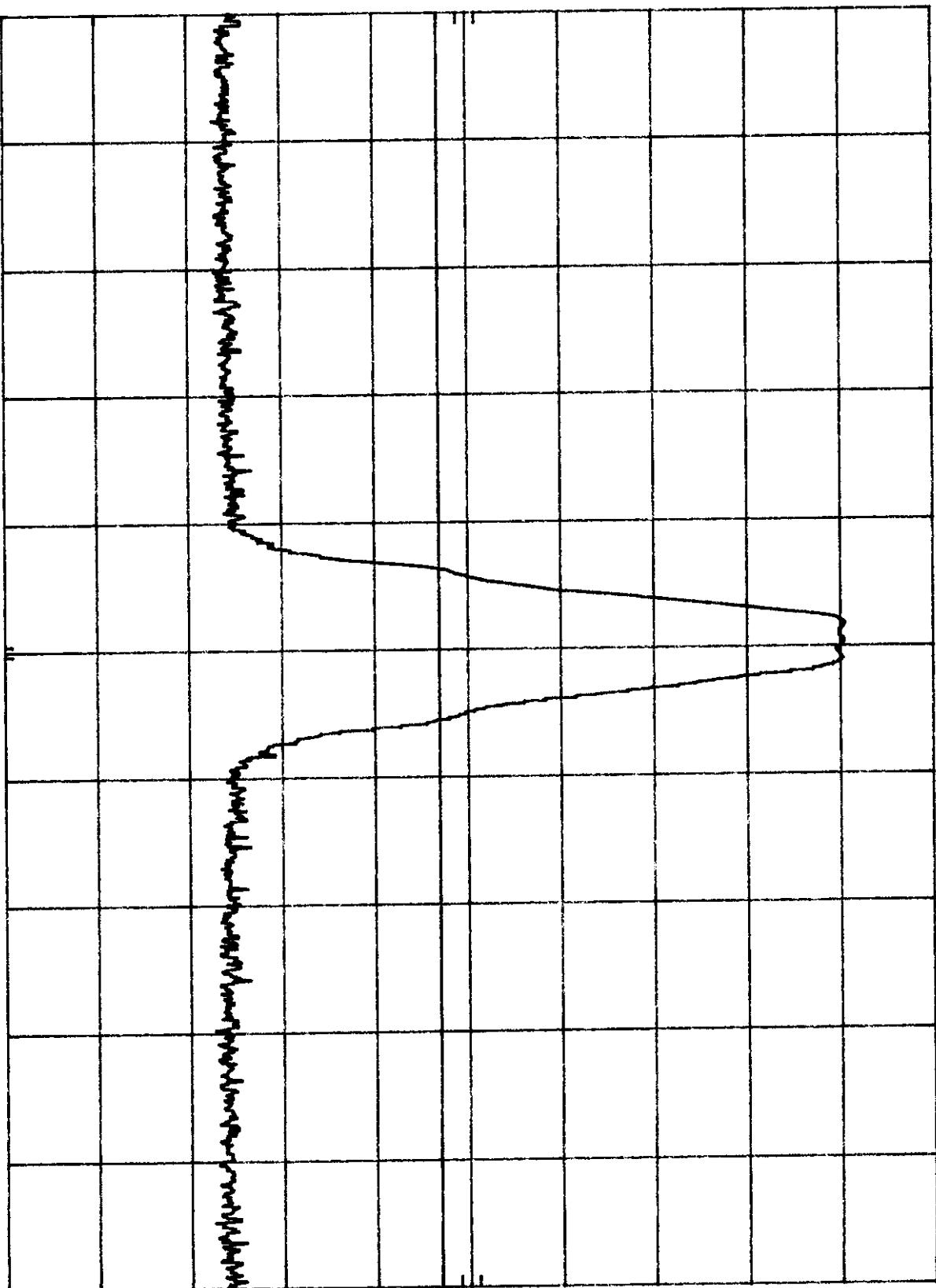
CENTER 932.02 MHz RES BW 100 kHz VBW 100 kHz
