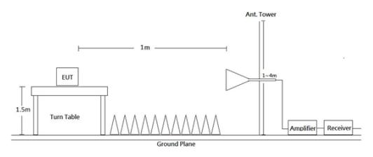
Radiated emission tests were performed in the 3 meters chamber test site, using the setup accordance with the ANSI C63.10-2013. The specification used was the FCC Part 15.209, FCC 15.247 and RSS-Gen, RSS-247 Limits.
