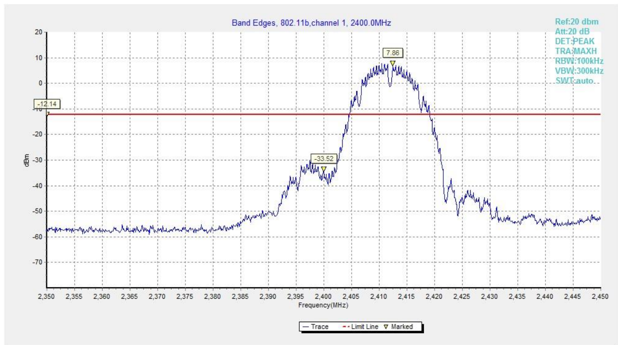
Fig.B.5.1 Band Edges (802.11b, Ch 1)
