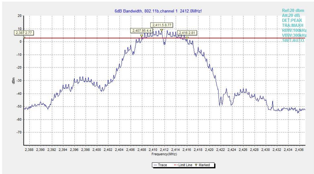
Fig.B.4.1 Occupied 6dB Bandwidth(802.11b,Ch 1)
