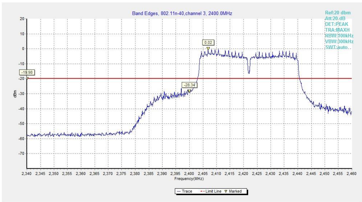
Fig.B.5.7 Band Edges (802.11n-HT40, Ch 3)
