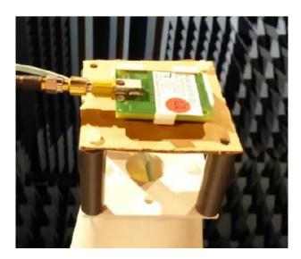
The gain values are at the technically possible maximum, in the 2.45 GHz band 2 and 3 dBi and in the 6 GHz band between 1.5 dBi and 4.5 dBi at the end of the band
