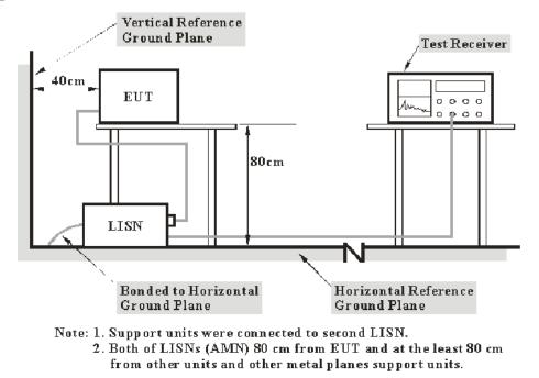
The measurement procedure of EUT setup is according with ANSI C63.10-2013. The related limit was specified in FCC Part 15.207 and RSS-Gen limits.
