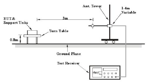
The radiated emission tests were performed in the 3 meters, using the setup accordance with the ANSI C63.10-2013. The specification used was the FCC 15.209, FCC 15.247 limits and RSS-247/RSS-Gen limits.
