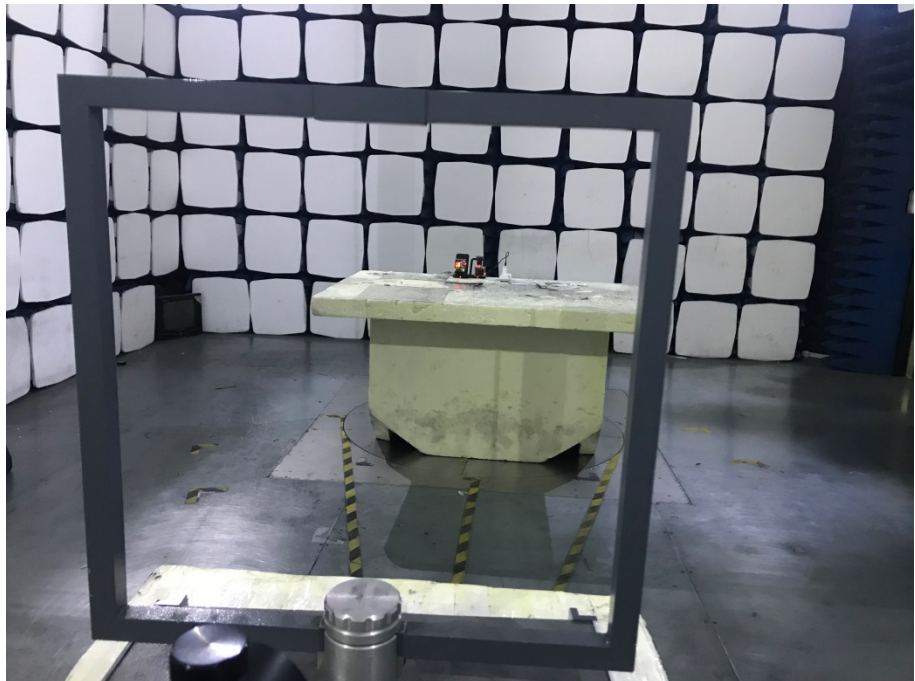
Radiation Emission Test Setup (Below 30MHz)
