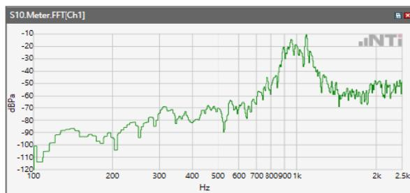
ANSI/TIA 5050-2018 \ 8N HAC OFF \ NB 12.2kbps\ 5.2 Receive path – distortion and noise\WCDMA Band V
