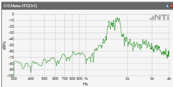
ANSI/TIA 5050-2018 \ 8N HAC OFF \ WB 23.85 kbps\ 5.2 Receive path – distortion and noise\WCDMA Band V
