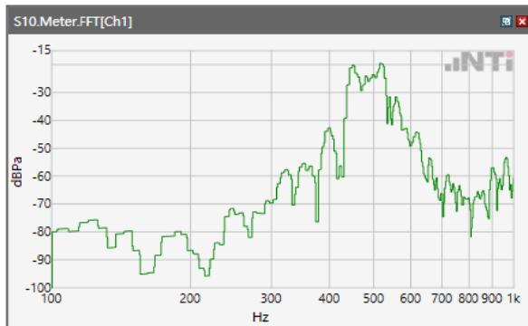
ANSI/TIA 5050-2018 \ 8N HAC OFF \ WB 23.85 kbps\ 5.2 Receive path – distortion and noise\LTE Band 2
