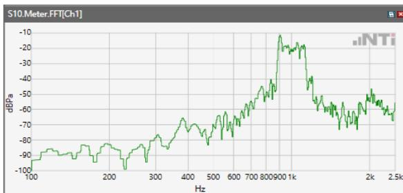
ANSI/TIA 5050-2018 \ 8N HAC OFF \ WB 23.85 kbps\ 5.2 Receive path – distortion and noise\LTE Band 2
