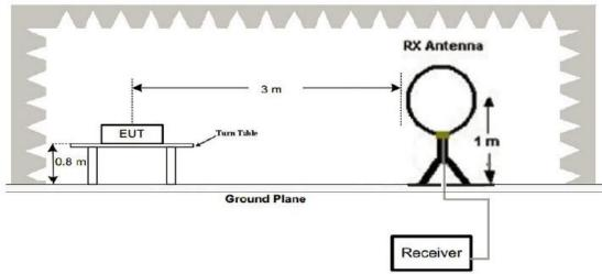
2. Radiated Emission Test-Up Frequency 30MHz~1GHz
